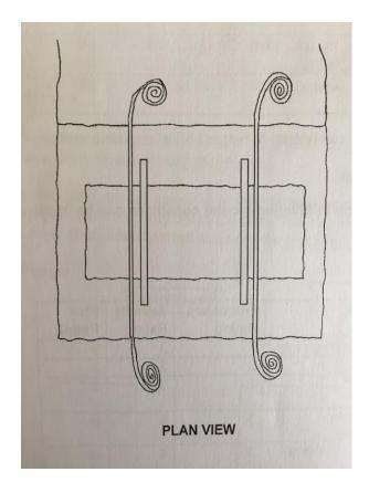
Two putlogs should be placed across the grave onto which the coffin may be placed prior to the committal. Putlogs should be 4'6" X 4" (1.37m x 102mm x 102mm) and of good quality knot free planed timber.
