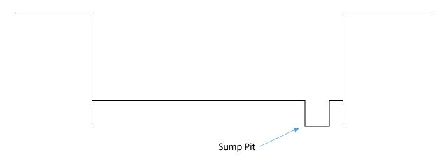
The hose from the pump can be placed in the sump pit and as water is pumped out of the pit the remaining water in the grave will be drawn towards the pit thus leaving the greater part of the bottom of the grave dry.
