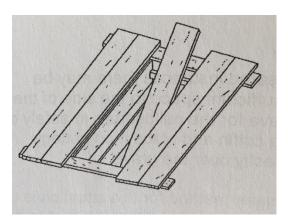
When backfilling large flints, pieces of rock or lumps of clay may damage the coffin when they impact from height. To reduce the risk of coffin damage a timber can be placed into the grave as shown in the above diagram. Backfill material will strike the timber, break its speed of fall and deflect to the sides of the grave.
