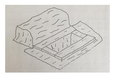
Grass matting can be draped into the grave to cover the internal walls and shoring equipment. The soil box, walkboards and immediate surrounding area can then be covered.
